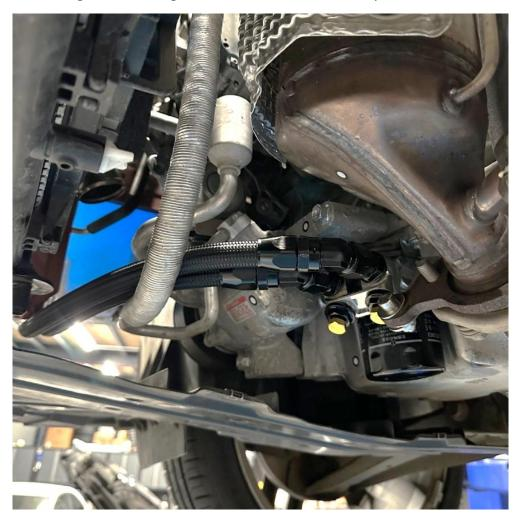
19. Fit the supplied oil line separators as shown to position the lines away from harm's way.
