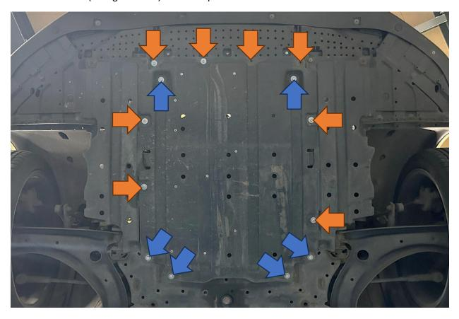
4. Remove the eight cross-headed screws (blue arrows) holding the bottom of the bumper to the car along with two plastic push fits (orange arrows).
