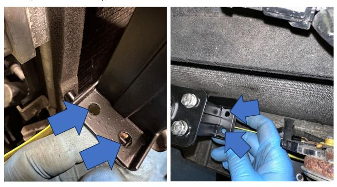
13. Now reinstall the plastic surround. Once in place, install the original plastic push fits except for the two holes where the lower oil cooler brackets are now located. For these, use the two supplied M6 Socket Head bolts with large washers to bolt through to the bracket, but do not fully tighten yet.
