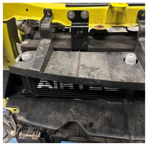
15. Now install the oil lines onto the oil cooler. The longer line with the 90-degree fitting goes onto the right-hand side and the shorter line onto the left-hand side. The lines route down next to the radiator, towards the engine.
