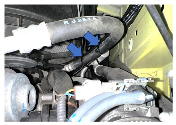
21. Finally, ensure all fittings are tight and then proceed to add 500ml of the correct grade oil to the car. Once added, start the car and check the fittings for any leaks and tighten as necessary. Stop the engine and once cool, check the oil level and top up as necessary. You can then refit the undertray and bumper in reverse of removal.
