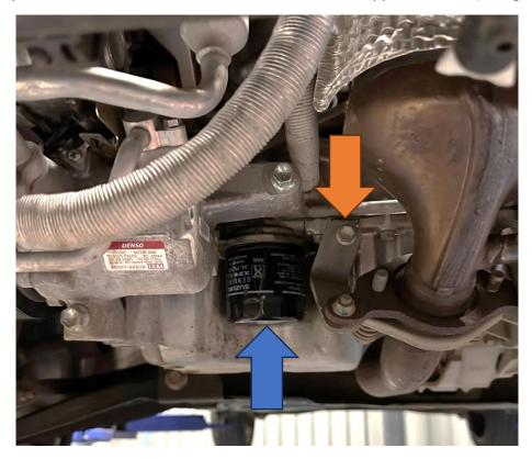
17. Install the supplied AIRTEC Motorsport exhaust support bracket. Once tight, install the sandwich plate adaptor onto the car and fully tighten the fitting so the take-offs are positioned as shown.
