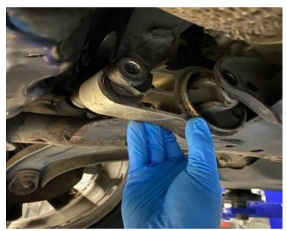
4. To fit the new torque mount, slide the supplied spacer shims into position on either side, as shown before fitting the mount into place.
