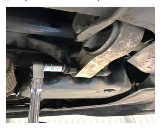
2. Now remove the 17mm bolt securing the other end of the torque mount in place.
