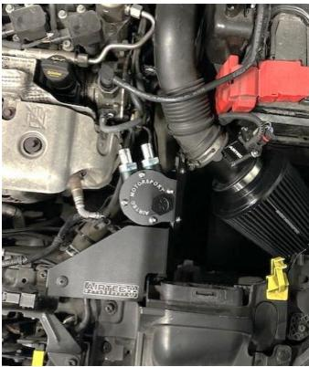
4. Locate the original engine breather recirculation hose (blue arrow) and remove it. Once removed, cut both connectors off from the middle tube section as you will be reusing them.
