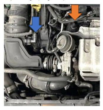
6. Finally, fit the two supplied hoses and route as shown. Secure the jubilee clips provided.
