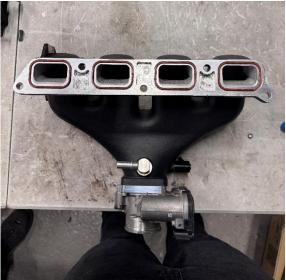
17. Position the manifold in place on the car without boltin it in place yet. Reconnect the silicone hose to the throttle body and tighten the jubilee clip. Then reconnect the wiring plug and the rear vacuum take-off.
