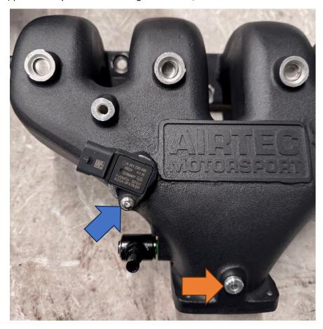
15. Now fit the supplied wiring harness bracket using the M8x12mm Socket Head bolt and washer provided.
