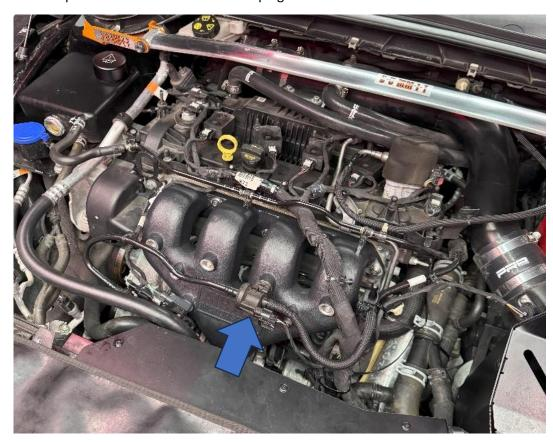
20. To refit the engine cover, install the supplied pins onto the new mounting brackets provided, as shown and then install onto the car using the M5 bolts with washers supplied.
