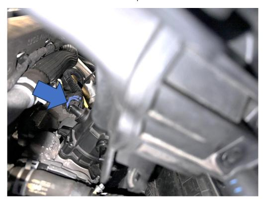
9. You can now access the wiring plug for the throttle body. Pull back the clip to release it, before squeezing so that it comes away. Once free, the inlet manifold can be removed from the car.
