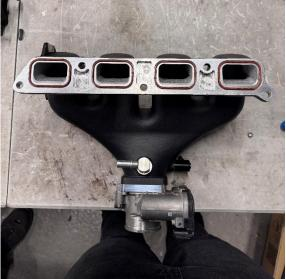
17. Position the manifold in place on the car without bolting it in place yet. Reconnect the silicone hose to the throttle body and tighten the jubilee clip. Then reconnect the wiring plug and the rear vacuum take-off.
