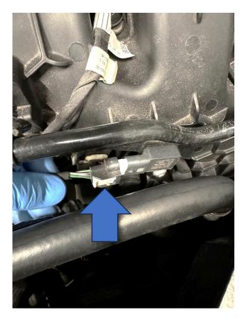
4. Remove the clip from the vacuum hose on the side of the manifold and then you will be able to push the other side of it in to release it, unhook it from the bracket and clip on the side. You will be able to then move the vacuum hose out of the way.
