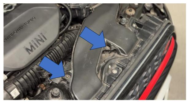
2. Release the MAF sensor by removing the two bolts securing it in place and then unplugging the wiring connector. Then loosen the jubilee clip securing the intake pipe to the air box using a 7mm socket and unclip the wiring loom attached to the air box (orange arrow).
