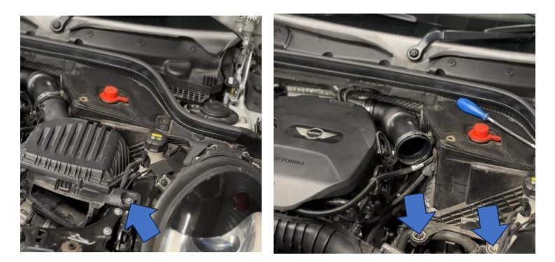
4. Now you can remove the original intake pipe by releasing the retaining clip, as shown below.
