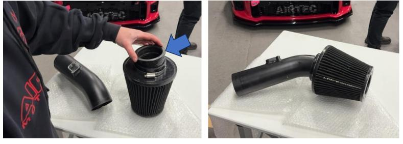
6. Install the supplied 80mm silicone hose with jubilee clip onto the original crossover pipe, but do not tighten to allow adjustment later on.
