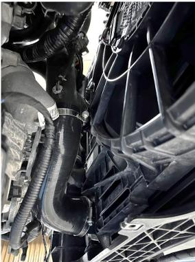
6. Working on the other boost pipe now, undo the jubilee clip attaching the silicone hose to the intercooler. Then remove the protective cap and undo the jubilee clip attaching the rear hose to the hard pipe.
