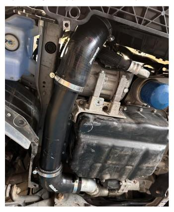
12. Finally, with all jubilee clips fully tightened you can reinstall the undertray, engine cover and induction hose.
