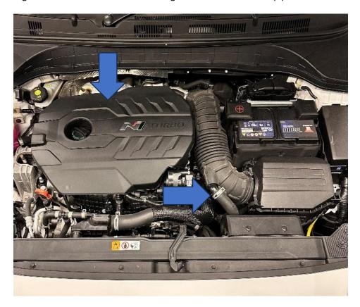
2. Remove the protective cap on the jubilee clip and then loosen the pipe to the throttle body.
