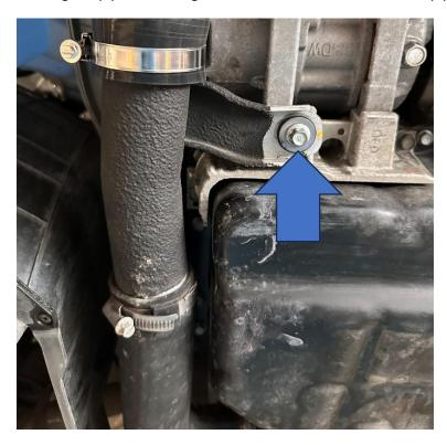
8. The original MAP sensor and recirc-valve need to be removed from the original pipe by undoing the 10mm bolts attaching them to the standard pipework (please note, this car is fitted with an aftermarket replacement recirc-valve so has 5mm Allen Key bolts instead).
