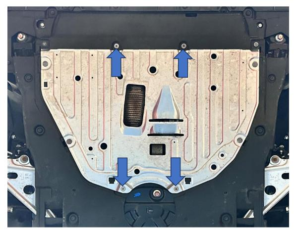
2. Next, undo the four rotation clips in each corner of the under tray. Then pull backwards to release it from the two plastic clips at the bottom and remove the undertray.
