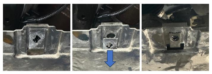
4. Now fit the new under tray in place making sure to reuse the two clips at the bottom. Secure in place using the eight supplied M6 Button Head bolts with washers.
