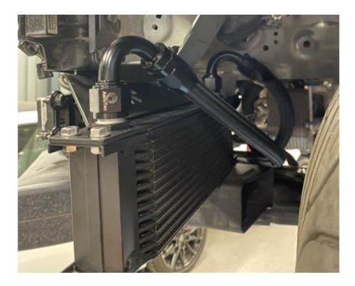
10. Using a suitable container to catch any oil, remove the oil filter from the car and then install your thermostatic sandwich plate using the supplied adaptor. Install the other ends of the oil lines to the sandwich plate and tighten. Before installing, smear a small amount of clean oil around the seal and then before installing a new oil filter do the same.
