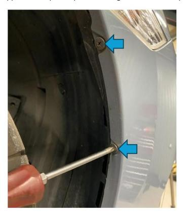
4. Release the two clips above each head light by inserting a pick tool inside the square gaps and pressing down.
