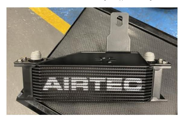
8. Locate the 17mm bolt on the right-hand side lower wheel arch. Remove it and then attach the oil cooler bracket to the car using the two supplied 10mm spacers. Then replace the original bolt with the supplied M8 bolt and washer, placing it through the bracket and into the hole, as shown.
