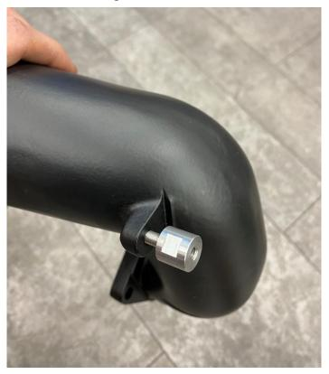
8. Transfer the gasket from the original crossover onto your new AIRTEC Motorsport crossover and then fit to the car reusing the original bolts. You can then bolt the wiring loom back onto the crossover using the original fixings.
