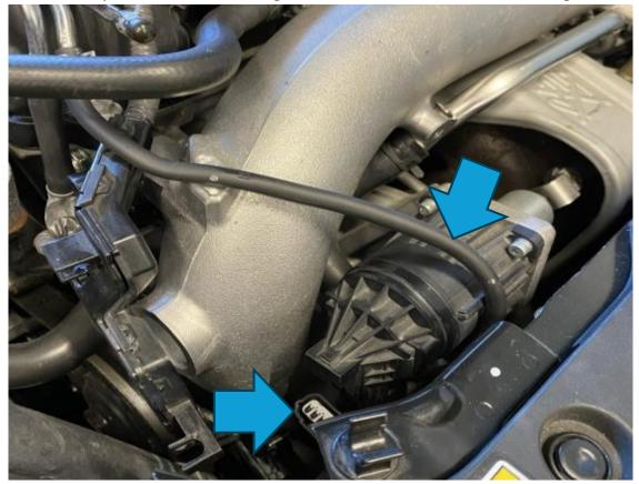
6. Undo the two 12mm bolts holding the crossover to the turbo and then lift it out the engine bay. Make sure to retain the gasket as this will be reused when fitting your new crossover.
