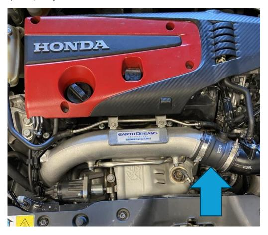
2. Undo the two 8mm bolts and two 10mm bolts holding on the pipework to the original crossover.
