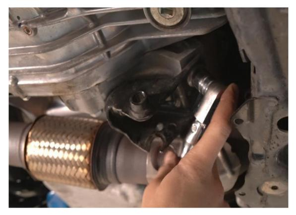
6. Install your new AIRTEC Motorsport torque mount by rocking the engine forward then reinstalling the bracket when in position.
