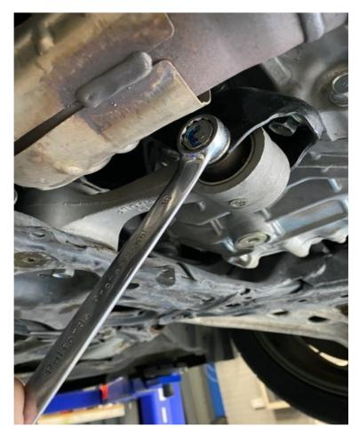
4. You can now remove the mount by rocking the engine forward.
