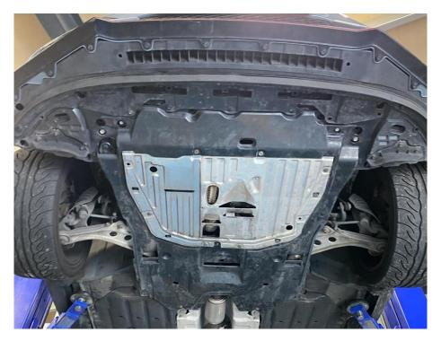
2. You will now be able to access the original torque mount, start removing the mount by removing the 17mm bolt securing the mount to the subframe.
