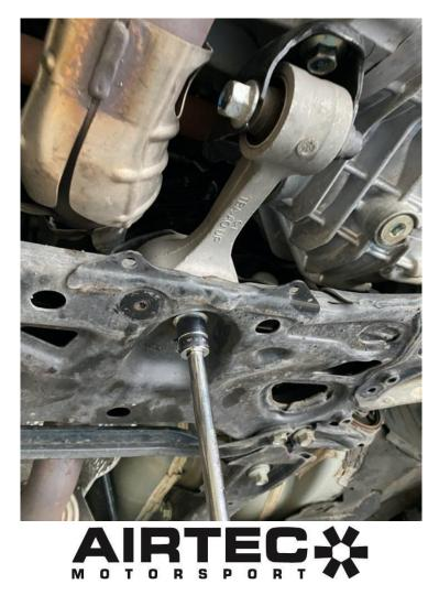
3. Now remove the 19mm bolt securing the lower mount to the bracket.
