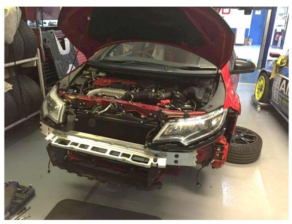
12. Before fitting the new intercooler, use the supplied bolts with washers to secure the locating pins provided to the bottom part of each mounting bracket, as shown. **Do not fully tighten to allow movement.**
