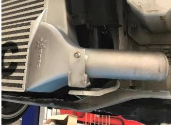
14. At the top of the intercooler, use the two supplied bolts with washers to secure and then refit the crash bar.
