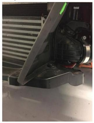
8. Now remove the two 10mm bolts securing each intercooler mounting bracket in place.
