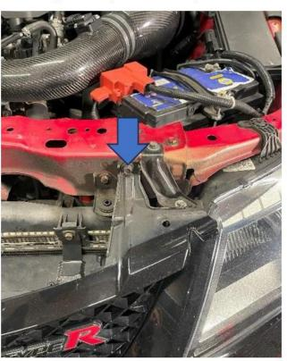
6. With the help of another person, carefully but firmly pull the bumper away from the car. Once the bumper is free do not fully remove it as there are still wiring connectors to disconnect. Reach inside the bumper and undo the parking sensor clips and fog light wiring connectors. The bumper will now come away from the car and can be safely put aside to work on – see next step.
