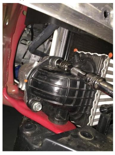
10. Undo the left-hand side boost pipe mounting brackets and remove the cast pipe together with the connecting silicone hose.
