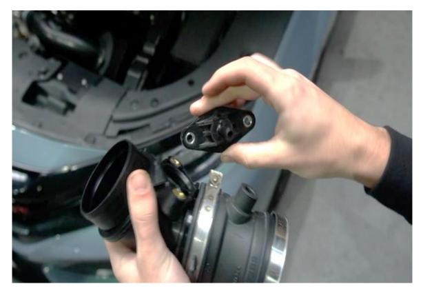
12. Now reinstall the vacuum line feed into your new pipework reusing the two 10mm bolts and then reconnect the vacuum line in reverse of removal.
