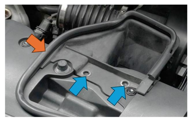
6. At this point we can remove the air guide from the engine bay.
