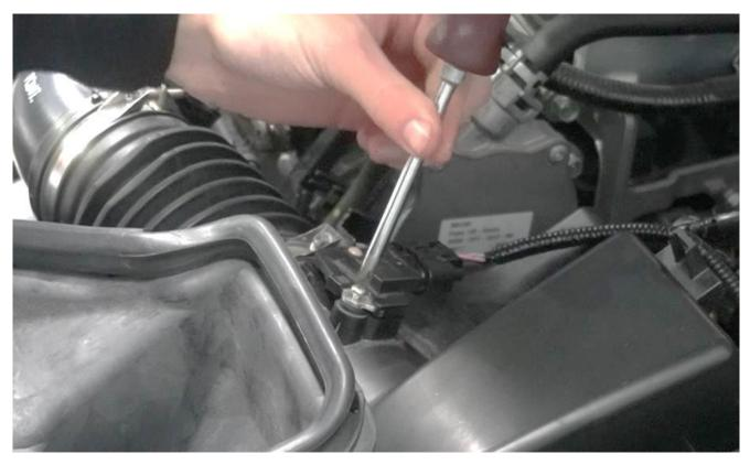
2. You can now loosen the jubilee clips securing the intake pipework in place.
