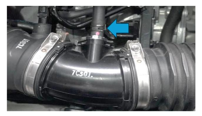
4. You can now remove the intake pipework.
