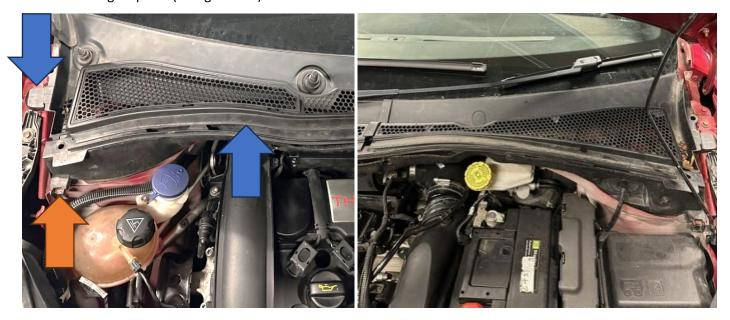
4. The lower scuttle panel is secured using two 10mm bolts on the outer edge (blue arrow) and two 10mm nuts in the centre (orange arrows).
