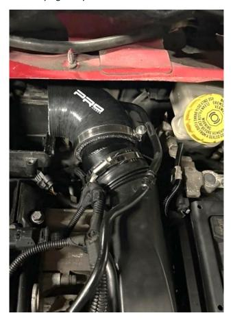
12. Fit the original MAF sensor to the supplied MAF housing plate pipe using the provided M6x16mm bolts, with Nyloc nuts and washers both sides, as shown.
