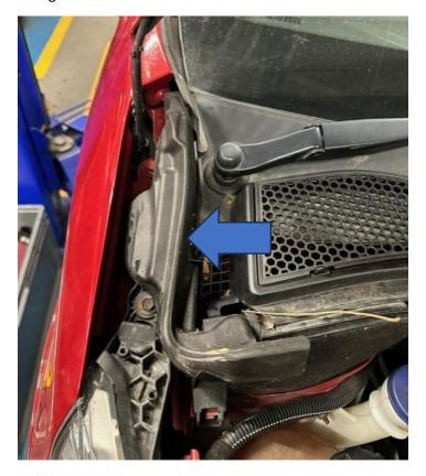
2. Remove the plastic caps from the wiper arms bolts with a small trim removal tool. Then use a 16mm socket to undo the nuts and pull the arms up to remove them from the splines.
