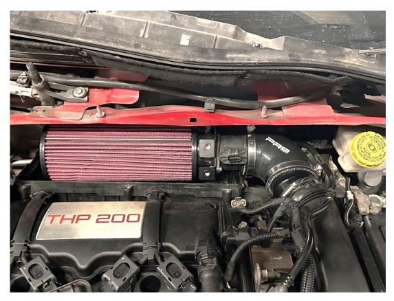
14. Use the supplied aluminium spacers with the original screws to secure the new lid in place. Once in place, tighten down all the jubilees.
