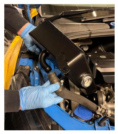
4. Hook the rear of the header tank over the clip first.
