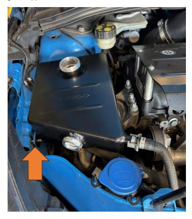
6. Finally, fill the tank with coolant. **Please note:** the level **MUST** go to the **TOP** of the sight glass, as shown.
