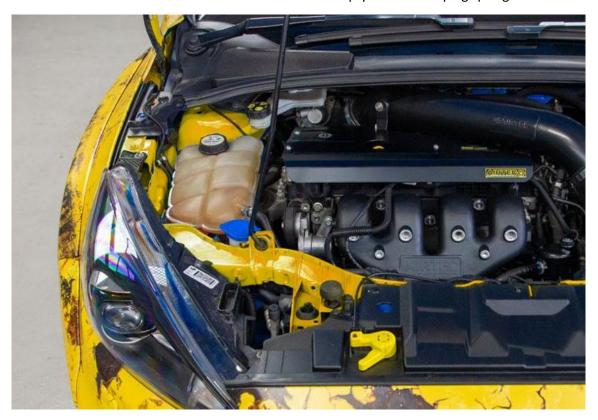
2. Before fitting the new AIRTEC Motorsport header tank, fit the supplied rubber push fitting that comes in the fitting kit into the boss on the bottom of the tank, as shown.
