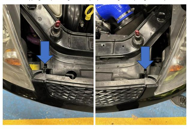
2. Locate and remove the 10mm screws inside the wheel arch on each side of the bumper. Then where the bumper meets the wing, carefully but firmly pull down to unclip both parts
