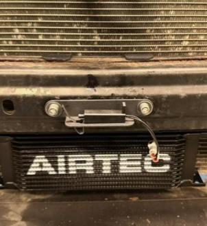
6. Working under the car, locate the oil filter and remove it. Be ready to catch any spillage. Then install the supplied AIRTEC Motorsport sandwich plate with the supplied fixing before fitting the oil filter.
