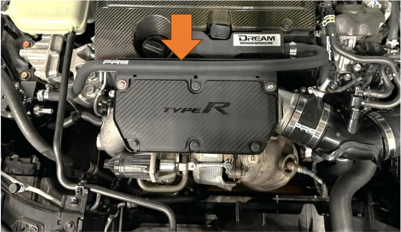
9. Place the second hose in the same location and connect it to the induction hose take-off fitted in Step 5. Secure both hoses with the supplied jubilee clips.
