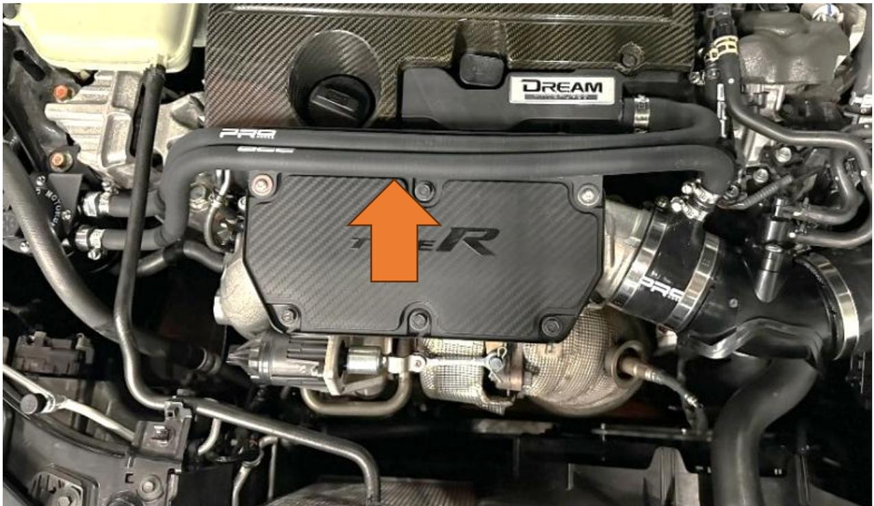
10. Secure both hoses to the mounting bracket fitted in Step 4 using the supplied cable ties. Make sure all jubilee clips and brackets are tight.
