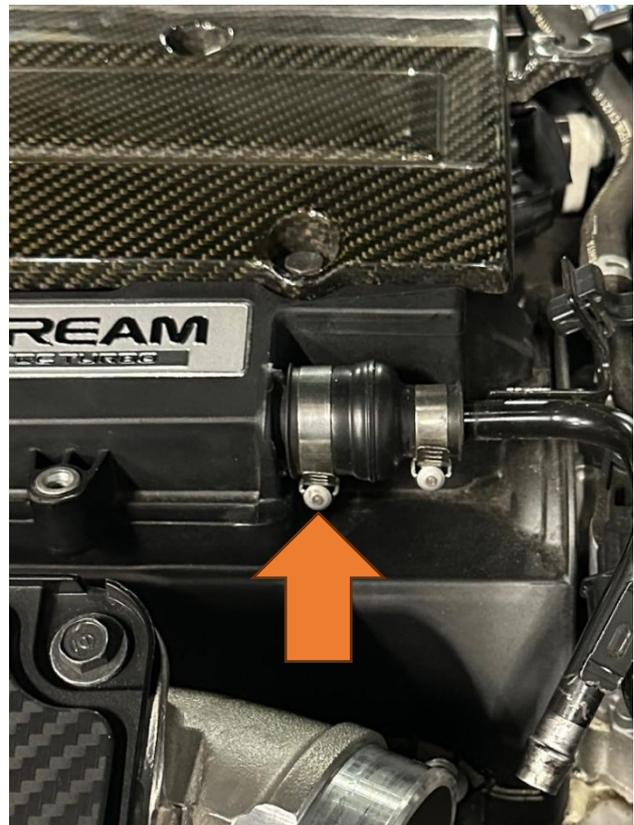
3. Prepare the small supplied silicone hose by pushing in both hose connectors provided and securing them with jubilee clips. Place an absorbing material under the hard pipe and remove both clips. Replace the hard pipe with the silicone hose and reattach the original clips. Hold it in place with a cable tie, as shown.
