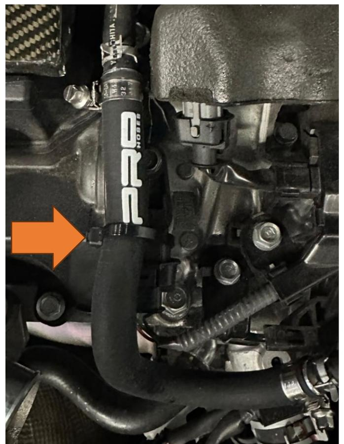
4. Locate the induction hard pipe and remove both the top left and right securing bolts. Fit the supplied billet spacers in their place and then secure the hose bracket in place with the provided bolts and washers.
