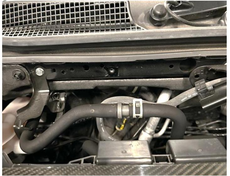
2. Locate the original breather hose at the back of the engine and release the hose clips securing it at either end to remove it. You can unclip the wiring loom on top of the engine for more clearance if required.
