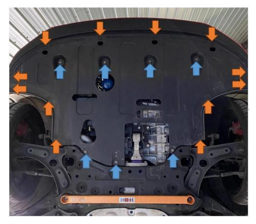
2. In both wheel arches there are three plastic clips that need to be removed using a trim tool and then an 8mm bolt.
