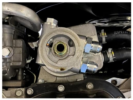
10. Attach the oil lines to the oil cooler ideally using an AN-10 aluminium spanner, which is recommended in order to avoid damage to the finish on the hose connectors. However, an adjustable spanner can be used but it is recommended to put some electrical tape around the connectors to minimise the risk of scratching. You can then fit the oil filter.
