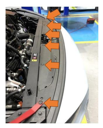
4. The edges of the bumper can now be carefully but firmly pulled out, which is best done by pulling from the top corner where the bumper meets the front wing and working your way forward. This is best done with another person doing the same on the other side so that once both sides are pulled forward one person can support the bumper whilst the other disconnects the wiring connector on the near side, which will be revealed when the bumper is ready to come off.
