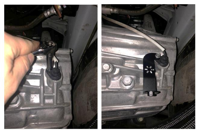
12. Attach the supplied line separator to the lines and secure it to the bracket. You can then feed the lines out in front of the arch liner and above the brake cooling duct.
