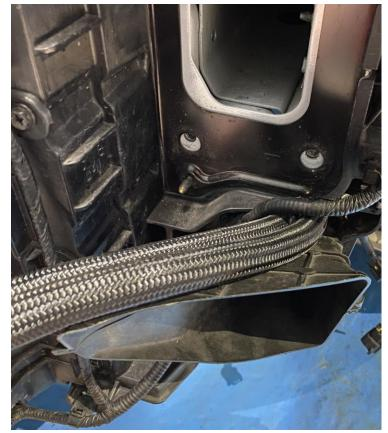
14. Attach the lines to the cooler in the same way they were connected to the sandwich plate and then refit the crash bar.
