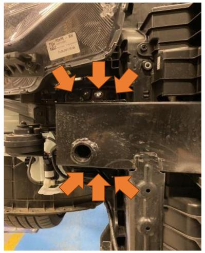
6. Divide the brackets into left and right-hand sides. Then, measure out exactly 240mm from the left-hand side of the crash bar and attach the left-hand bracket by hooking the larger part under the crash bar and pushing it up so that it clips onto the front of the bar.
