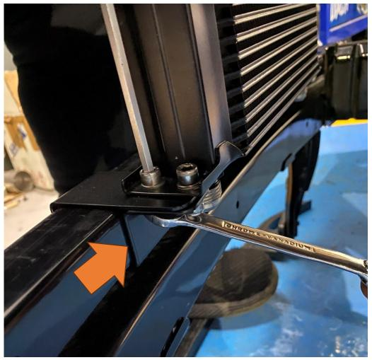
8. You can now fit the right-hand side bracket in the same way and once fully tightened, refit the crash bar to the car.
