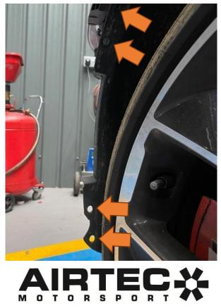
3. . There are six plastic clips to be removed with a trim tool along the slam panel.
