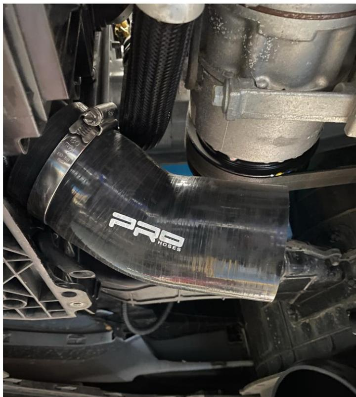
14. Fit the new pipe into the silicones and get it into a position where it fits well at both ends and the bracket lines up with the original mounting hole.
