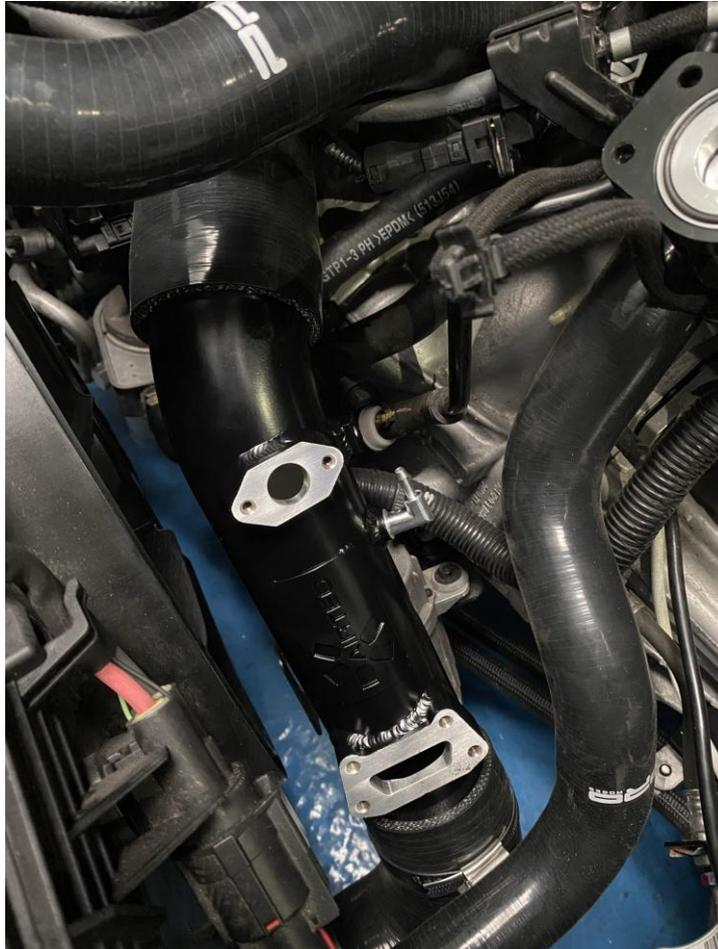
17. You can now build back up the cold side pipe by attaching the MAP sensor to the pipe using the supplied M5x12mm with washers, reconnect the plug, attach the solenoid to the mount reusing the original bolt and attach the vacuum line to the take off and secure with the original clip.
