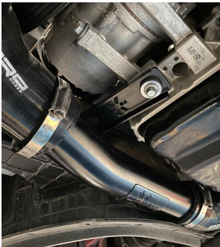
15. Tighten the bracket onto the car reusing the original bolt and then tighten the M6 holding the bracket to the boost pipe and tighten all the jubilees once happy with the positioning. Work from the top or bottom fit the new silicone that comes from the intercooler to the new large cold side pipe.
