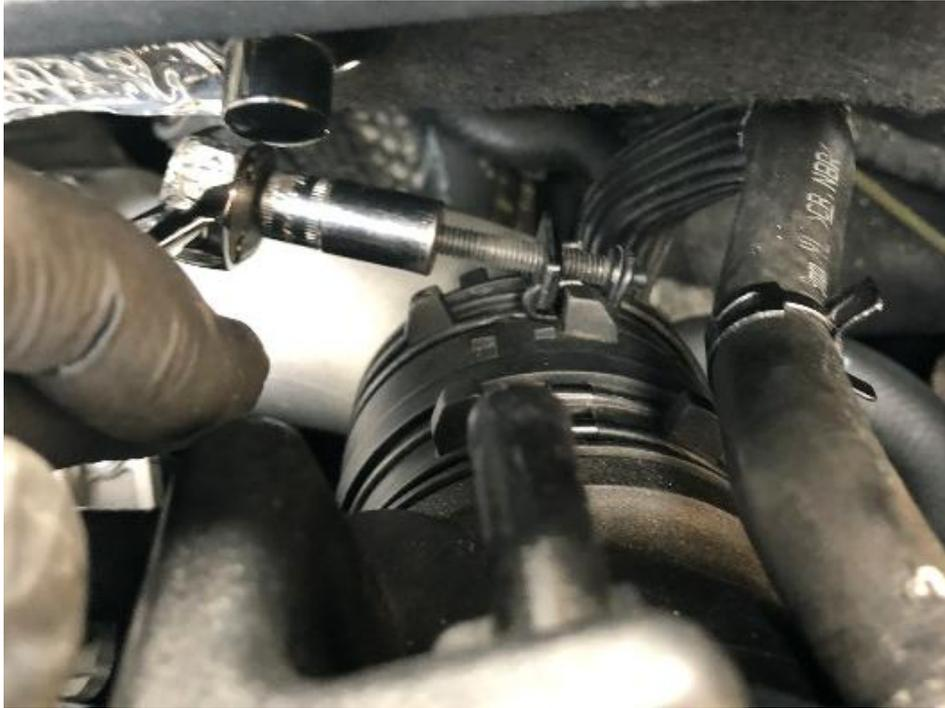
2. Unclip the two breather hoses on top of the induction pipe at the back of the engine bay and also the clamp holding on the hose at the front on the induction pipe by squeezing the clips with a pair of pliers and pull the clamp down the hose. The hoses can then be removed by pulling the hoses off the original pipe.
