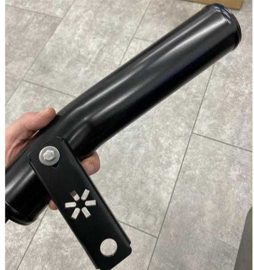
13. Loosely fit the two silicones into place with jubilee clips, but do not fully tighten at this stage. One will be a 90-degree from the original turbo hard pipe and the other is a shallow bend. There will be one that suits the standard intercooler and one that suits the AIRTEC Motorsport intercooler. Use the correct one to suit your application.
