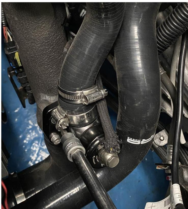
5. The MAP sensor will need removing, firstly unplug the connector and then remove the two 10mm bolts holding it to the pipe.
