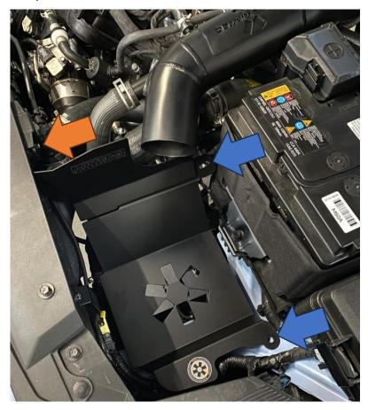
12. Install the filter onto the trumpet and then fit the supplied silicone connector onto the trumpet and tighten the jubilee clips. This can then be installed onto the car.
