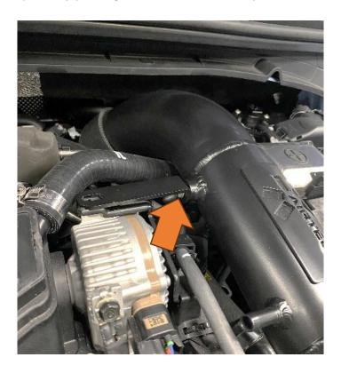
8. Tighten the rear jubilee clips and then refit the bolt removed in Step 6 to secure the mounting bracket. Fully tighten the mounting bracket bolt to the pipe and then reattch the two pipes removed in Step 2.
