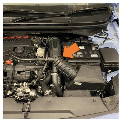
2. To remove the induction pipe, loosen the two hose clamps highlighted below using pliers and then disconnect the hoses.
