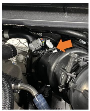
4. Undo the three 10mm bolts securing the air box (orange arrows). Then remove the two 10mm bolts holding the front air feed in place (blue arrows). You can then remove the assembly from the car.
