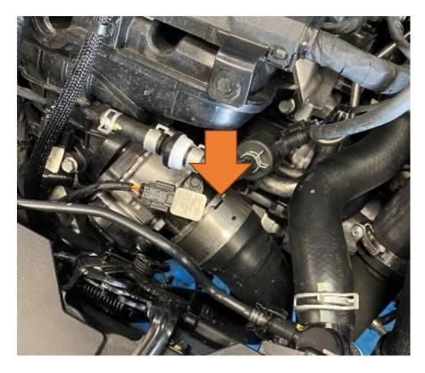
4. Remove the MAP sensor by undoing the 8mm bolt securing it.
