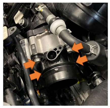
6. Take the gasket from the throttle body flange and install it onto your AIRTEC Motorsport throttle body adaptor. Then install onto the car reusing the original bolts.
