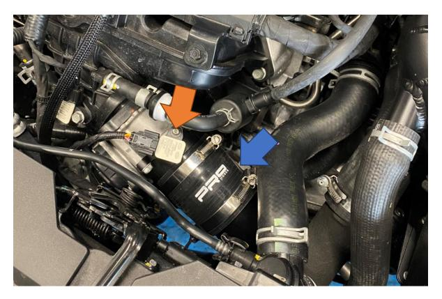
8. Install the bracket onto the supplied boost pipe using the supplied M6 bolt and washer, but do not fully tighten to allow adjustment.
