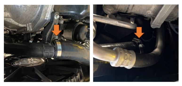
2. Now remove the 10mm bolt holding the boost pipe to the gearbox.
