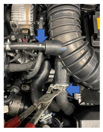
6. Undo the two 10mm hose clips at either end of the intake pipe and remove it from the car.
