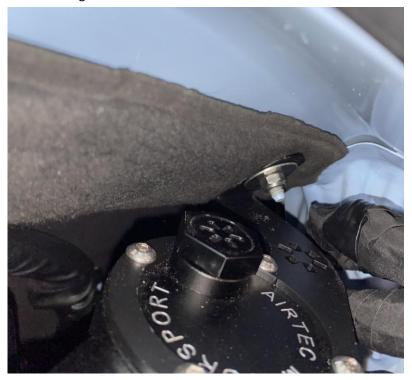
10. Now install the hoses. The shorter hose goes from the catch can to the connecter removed in Step 2. The longer hose goes from catch can to the connector removed in Step 4, as shown.
