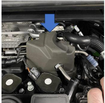
4. Using hose clamp pliers, release the back hose clip and disconnect the pipe. This can now be removed from the car.
