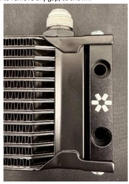
12. Mount the oil cooler to the car using the supplied M8 bolts to go through the mounting blocks to the brackets installed earlier. Once happy with the positioning ensure all the oil cooler bolts are tight.
