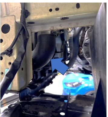
11. Secure the upper part of the radiator assembly on both sides using cable ties in a suitable place, as shown.
