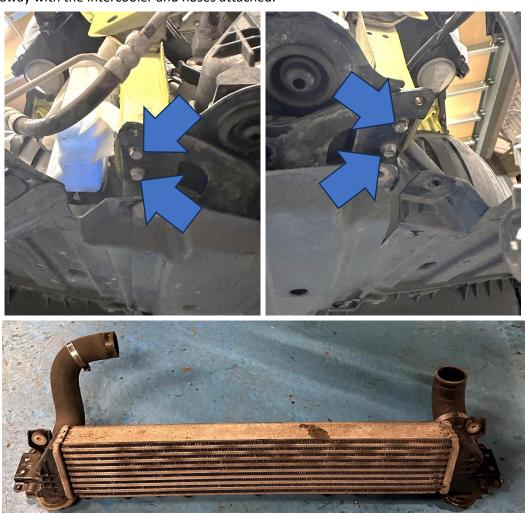
15. Install your new Pro Hoses silicone hoses with jubilee clips but leave them loose before lifting the new intercooler into place and reusing the two bolts removed in Step 13.
