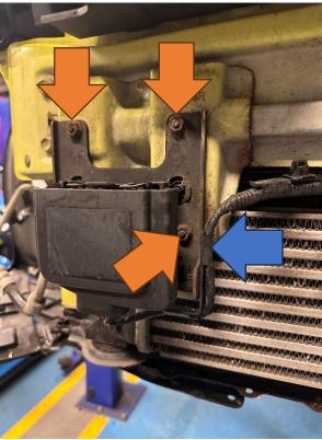
13. Undo the two 10mm bolts holding the top of the intercooler in place.
