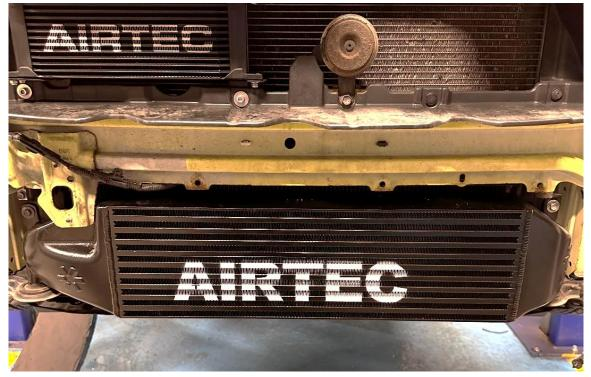
17. Install the supplied temperature sensor relocation bracket on the right-hand side using the supplied M6 bolt and washer and then clip the wiring harness and sensor in as pictured.
