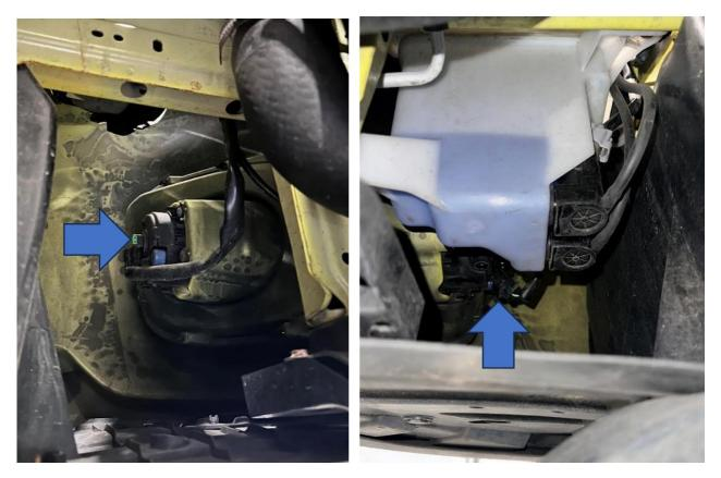
6. Using a second person to help, release the bumper by firmly but carefully pulling the corners before lifting the centre and pulling it away from the car. You can then place it safely aside.
