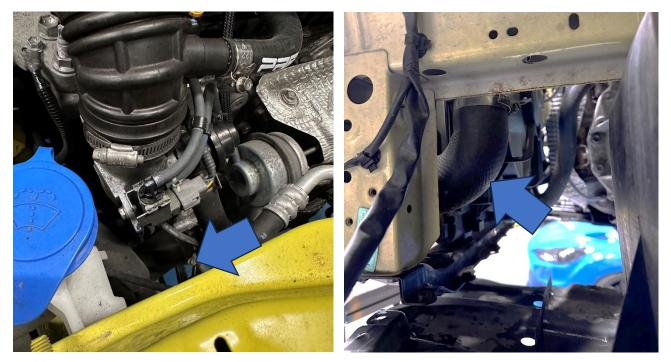
11. Secure the upper part of the radiator assembly on both sides using cable ties in a suitable place, as shown.
