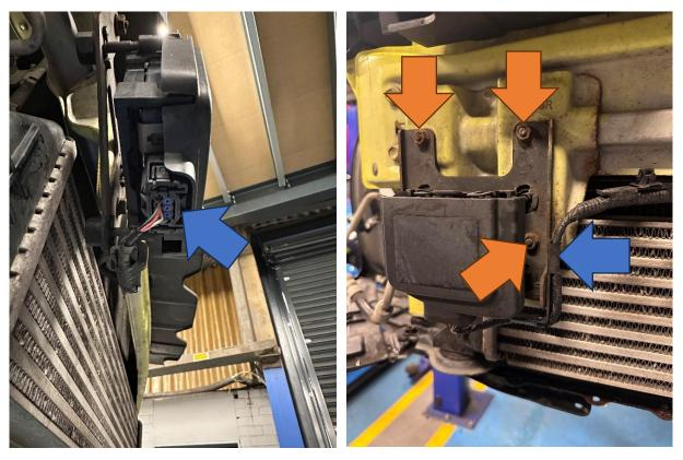
13. Undo the two 10mm bolts holding the top of the intercooler in place.
