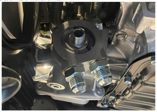
16. Now install the oil lines. The shorter line goes to the left-hand side of the cooler and feeds through underneath the headlight to the sandwich plate fitting nearest the front of the car, as pictured. The longer one goes from the right-hand side to the rear sandwich plate fitting.
