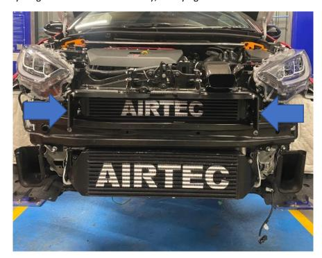
18. Finally, top up the oil and start the car. Look immediately for leaks from any of the four connections and the oil filter. If so, turn the engine off and retighten the fittings if needed. Then let the car get to full operating temperature, recheck the oil level and top up if required.
