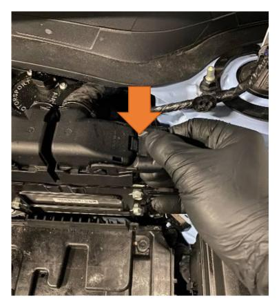
6. Undo the 10mm bolt holding the ECU in place on the left-hand side and then the two 10mm nuts holding the ECU to the strut tower.
