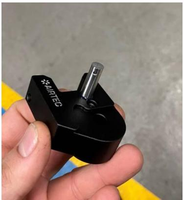
10. Now install the quick shift onto the shifter arm and secure in place using the original R-clip. Then apply the supplied thread lock to the grub screw and fit in place as shown.
