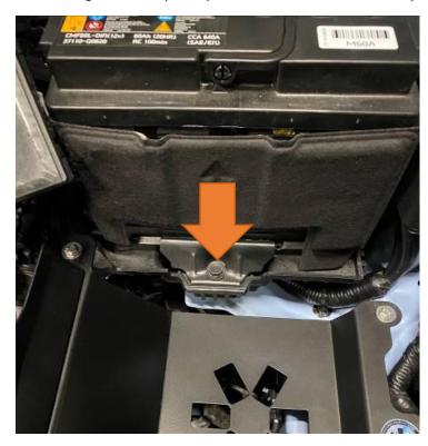
4. Remove the 10mm bolt that connects the induction shield to the battery tray, and the 10mm bolt holding the wiring harness down on the left-hand side of the battery tray.
