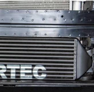
12. Install the provided bracket to the right-hand side of the crash bar with the supplied M6 fixings. Clip the temperature sensor in position as shown.
