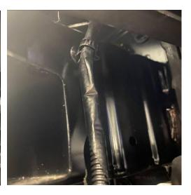
6. Remove the crash bar by undoing the four 12mm bolts (highlighted with orange arrows) and one 10mm nut (highlighted with blue arrow) each side.
