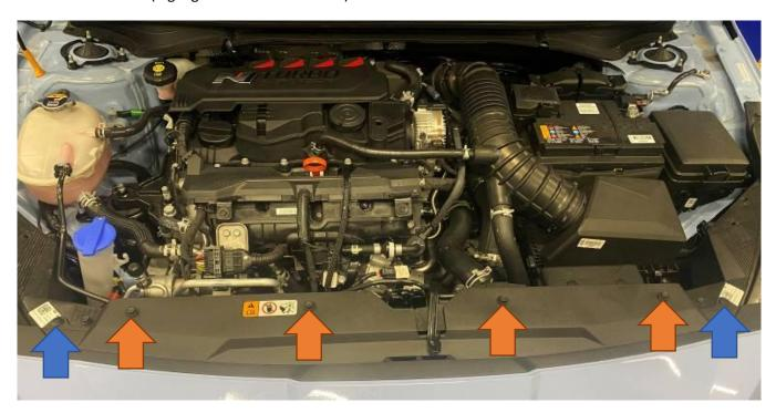
2. Working in the front wheel arches, remove the three trim clips (highlighted with orange arrows) followed by the 8mm bolt (highlighted with blue arrow) that attaches the front bumper to the wing on both sides.
