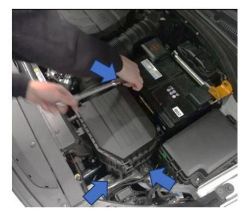
4. Undo and remove the cold air feed block that is attached to the front panel shown in the photo below, retain one of the bolts as this will be reused when fitting the new induction shield.
