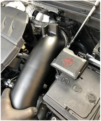
8. Using the supplied M6x12mm dome headed bolt and washer mount the bracket that was fitted to the block earlier to the boss on the side and tighten to hold the pipe securely to the bracket, leave the bracket itself still slightly loose at this point so the pipe can be positioned correctly once the filter is on.
