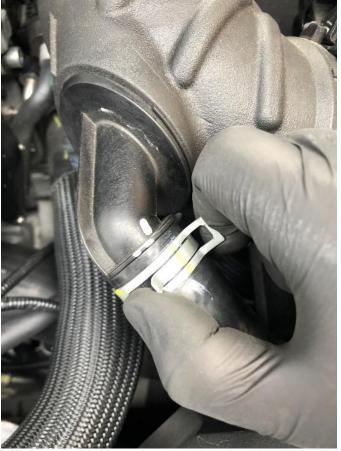
2. Undo the hose clamps at either end of the induction pipe there are undone using a 10mm socket, once undone the induction pipe can be removed from the car.
