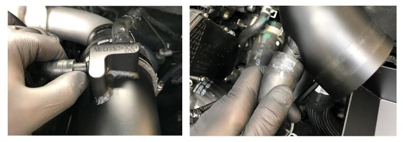
10. Attach the silicone reducer (100mm-90mm) onto the filter and tighten, then attach the reducer onto the induction pipe and position with the jubilee clips as shown in the photo below to ensure clearance between the heads of the clips and the shield and tighten. Tighten the bracket holding the pipe to the block once you are happy with the position of the induction pipe.
