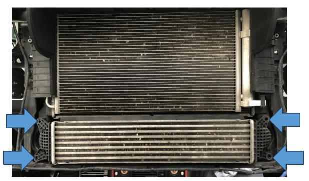
10. Before you can install your new AIRTEC Motorsport intercooler you will need to remove the temperature sensor bracket from the crash bar. This is best done using an angle grinder. We recommend painting over the cut on the crash bar to help prevent rusting.
