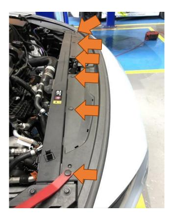
4. The edges of the bumper can now be carefully but firmly pulled out, which is best done by pulling from the top corner where the bumper meets the front wing and working your way forward. This is best done with another person doing the same on the other side so that once both sides are pulled forward one person can support the bumper whilst the other disconnects the wiring connector on the near side, which will be revealed when the bumper is ready to come off.
