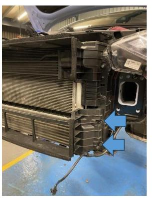
8. Undo the jubilee clips holding on both the boost hoses enough so that they are free to slide off. To remove them you will need a pair of grips or a flat-bladed screwdriver to remove the cap and then an 8mm socket to undo them. Remove both hoses from the car, as these are not used when installing your new intercooler.
