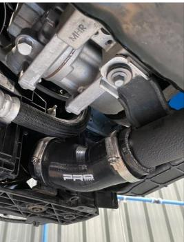
12. Install your new AIRTEC Motorsport intercooler by angling it in on the left side when looking at the vehicle from the front and then pushing the right side in place and secure in place by reusing the original 10mm bolts removed in Step 10.
