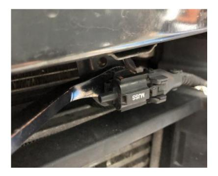
6. Remove crash bar by releasing the two 10mm nuts each side followed by the four 12mm bolts, then tilt the bar forward and pull out. This is best done using a second person to support the crash bar during the process.
