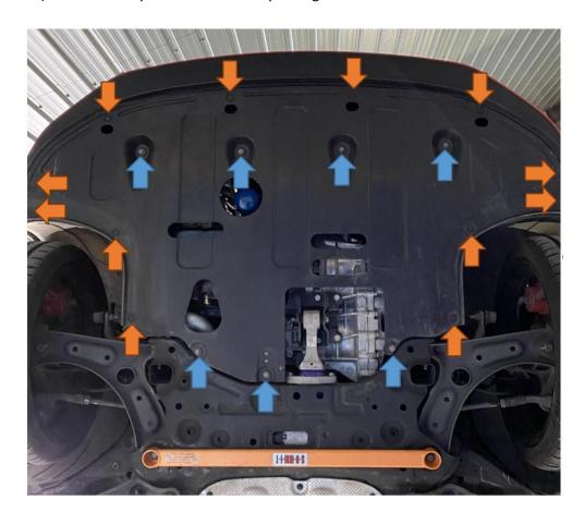
2. In both wheel arches there are three plastic clips that need to be removed using a trim tool and then an 8mm bolt.
