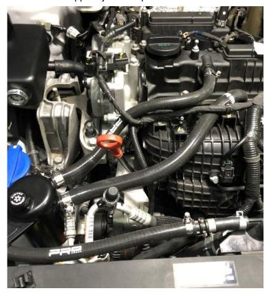
8. Finally, check all hose clips are tightened and then the engine cover can be replaced. Ensure it is fully seated by pushing down on each of the four mounting rubbers. Then check the coolant level and top up if required.
