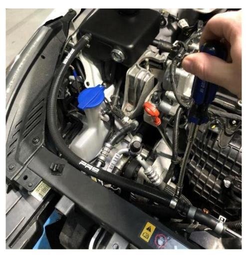
6. Remove the headlight bolt using a 10mm socket and then place the catch can in position. It will fit the profile of the headlight bracket which will help to locate it correctly so that it does not foul on the washer bottle lid. Refit the bolt when aligned correctly.
