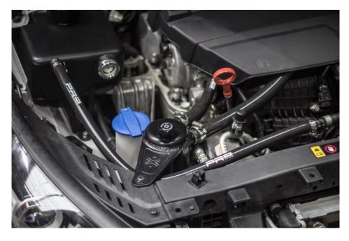
**Please note:** You should periodically check the oil level in the catch can using the provided dipstick. To drain the can, simply undo the jubilee clips holding on the hoses in place, remove the bolt attaching the bracket to the headlight and then tip upside down with the dipstick removed and allow to drain. Once drained, reinstall the catch can.
