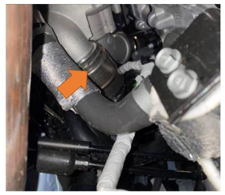
2. On the other end of the hose release the jubilee clip and then remove the connector.
