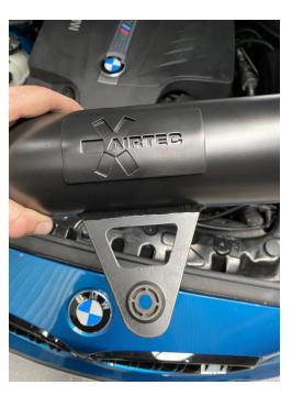
6. Pull up on the air box to release it from its rubber mounting and then remove the hard pipe and air box from the car as a whole.
