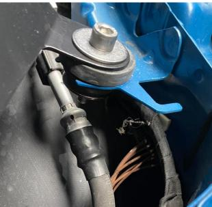
12. Reinstall the brace removed at the start and when happy with the position of the hard pipe fully tighten the original jubilee and bolt to firmly secure the induction kit.
