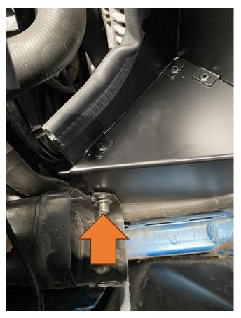
8. Remove the 13mm bolt on the slam panel highlighted and then place the alloy supplied spacer on top of this hole before fitting your new AIRTEC Motorsport intake pipe on top of it. Fit the pipe by guiding the filter end in through the hole in the air box and then push the other end into the original hose and then fix into position by reusing the original bolt to hold the pipe – but do not fully tighten yet.
