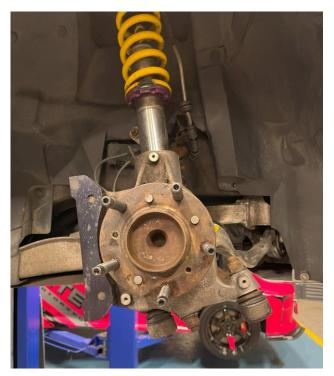
2. Slide the supplied backing plate on the correct side over the hub at its smallest point, as shown.
