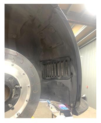
12. Route the ducting together along the control arm and use the supplied cable ties to secure tightly in place. **Please note:** It is advisable to fit a wheel back on and check to ensure that the hoses clear when the steering is on full lock in both directions. Re-adjust the hose routing if there are clearance issues.
