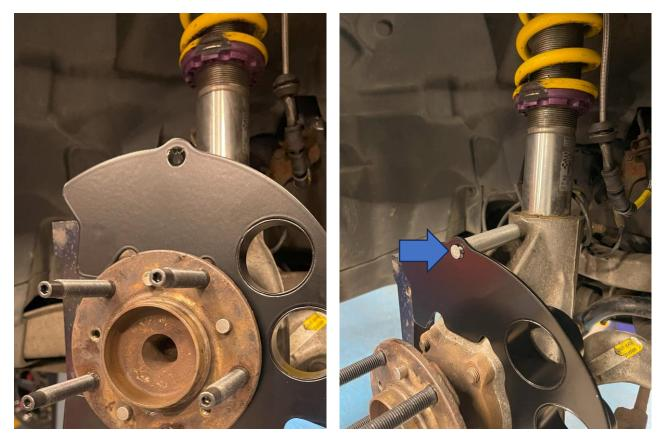
4. Now fit the shortest supplied spacer and bolt in the hole located nearest to the track rod end.
