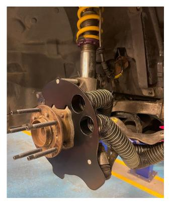
10. Now place a section of the supplied heat shrink shielding over each connection and join the two smaller hoses to the supplied brake duct divider. Use a heat gun on a **low setting** (or a hair dryer) to **slowly** seal the hoses to the duct divider. The larger remaining hose can be then added to the other end in the same way.
