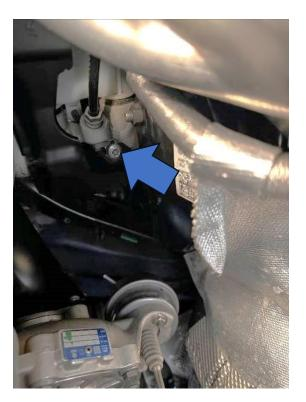
13. With the shield removed, mark out the section highlighted in blue and cut away using a suitable cutting tool. Then reinstall the shield onto the car.
