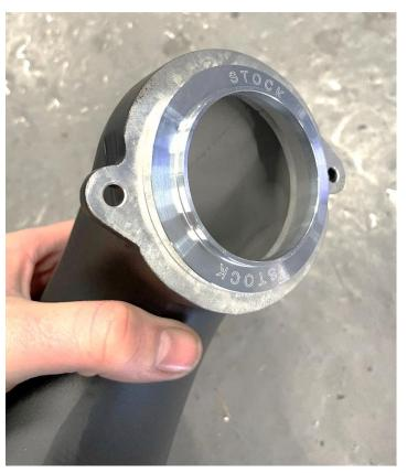
15. Now fit the new turbo elbow with the two supplied M6 bolts. Space is very limited to get the turbo elbow into position due to the increased size of the pipe, so be careful not to get it scratched when trying to install it. It is best to install it in the direction as shown and then rotate it into position once able.
