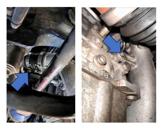
8. Remove the two T27 bolts holding the turbo elbow in place. The upper bolt (blue arrow) can be removed from above and the lower bolt (orange arrow) from underneath. The elbow can then be removed from above.
