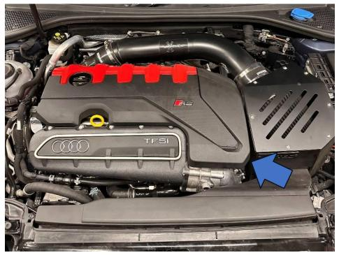
2. Remove the rear induction pipe. The car pictured is fitted with our AIRTEC Motorsport induction kit and so to remove the rear pipe you will need to undo the jubilee clips highlighted. Then unclip the vacuum line and undo the bolt holding the bracket to the engine.
