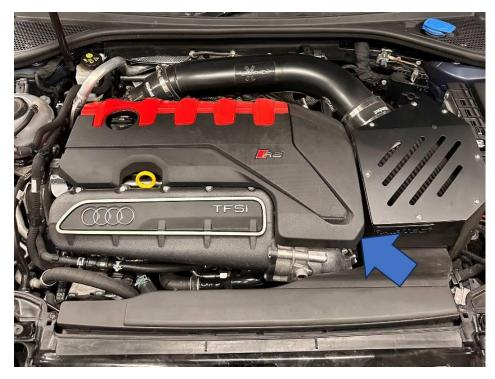
2. Unplug the wiring connectors going to the throttle body, recirc valve and both MAP sensors (blue arrows). You will need to remove the recirc hose (orange arrow) using hose clamp pliers to gain access to the lower MAP sensor plug. Once disconnected, move the wiring loom out of the way.
