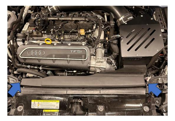
4. Undo the 10mm bolt holding the bracket highlighted onto the inlet.
