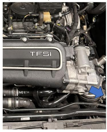
6. Undo the five 10mm bolts holding the upper and lower inlet plenum together. Using a rubber hammer, gently tap around the plenum to loosen the seal and **but do not remove it yet.**
