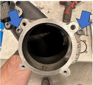
14. Install the supplied O-ring onto the new AIRTEC Motorsport cast elbow.
