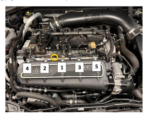
20. Install the supplied silicone reducer hose with jubilee clips but do not fully tighten to allow adjustment.
