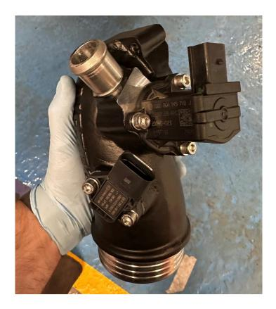
16. Also remove rubber bung from the top of the original elbow and install it onto your new elbow.
