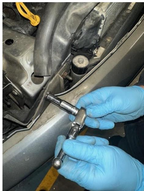
2. From underneath, remove the seven Phillips screws holding the lower front bumper in place.
