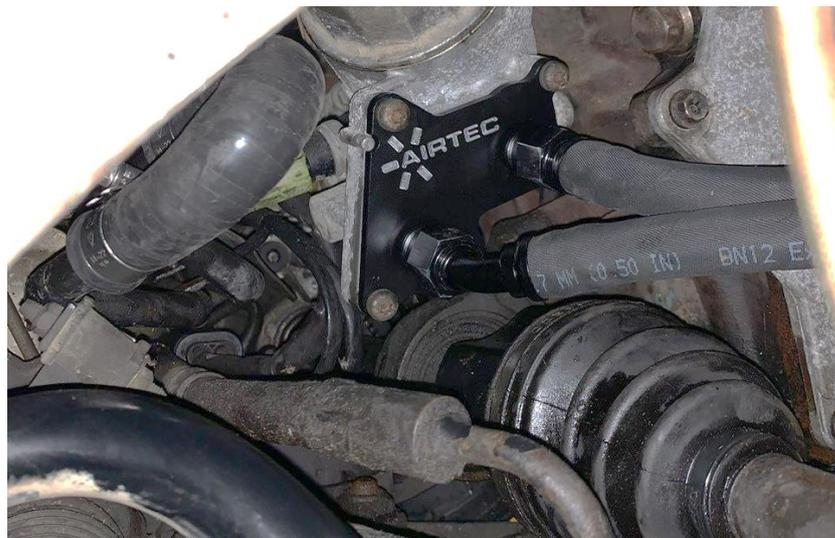
10. Run the lines past the crankshaft pulley and then pass them through in the gap below the fog light. Make sure there's plenty of slack so the lines keep close to the inside of the wheel arch but away from the pulley.
