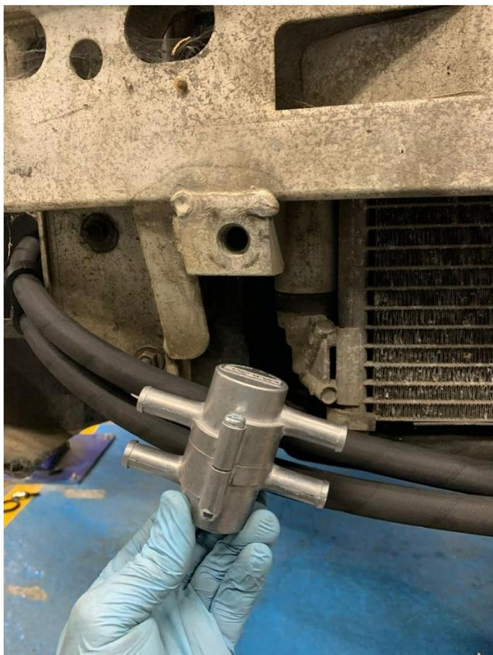
12. Now fit the bracket to the oil cooler using the bolts, washers and nyloc nuts as shown. Then attach the two remaining hose connections to the oil cooler and fully tighten.
