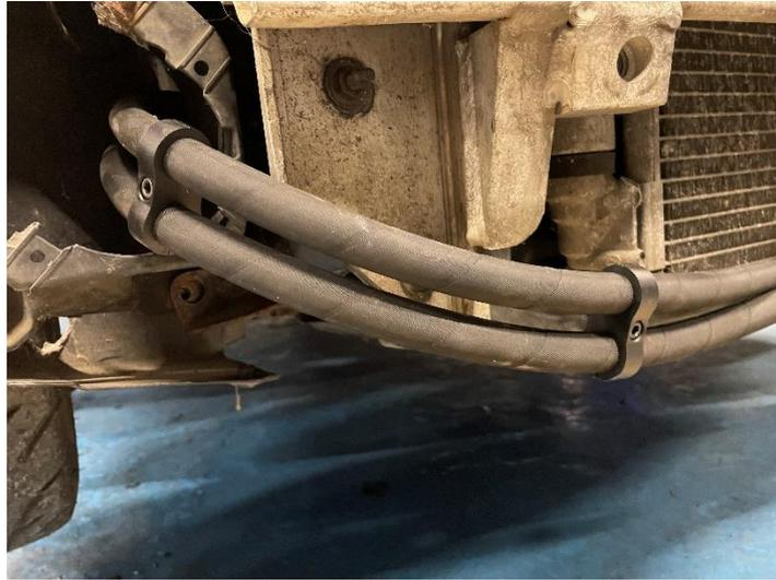
9. **IMPORTANT:** Finally, top up the oil and start the car. Look immediately for leaks from any of the connections. If there are, turn the engine off and retighten the fittings and repeat. Then let the car get to full operating temperature, let it cool and recheck the oil level and top up if required. The bumper, wheels and arch liners can then be refitted in reverse of removal.
