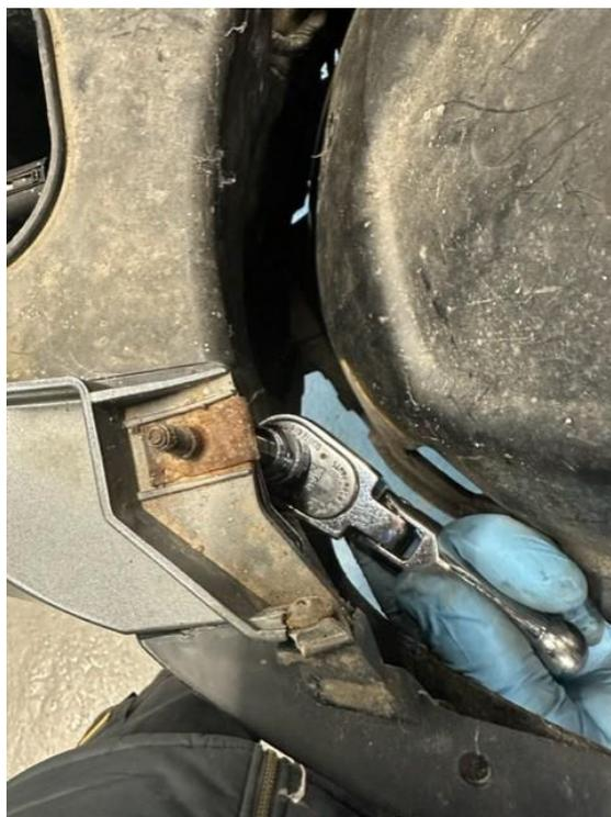
4. Now carefully pull the bumper off the top tabs to release it **but do not fully remove it yet.**
