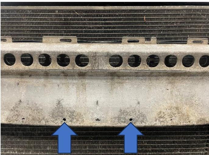
14. Now install the supplied M6 Riv Nuts and fit the oil cooler in place using the supplied bolts with large washers and fully tighten.
