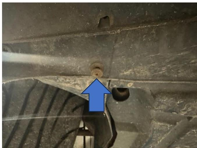
3. Remove the fixings inside the front of the inner arch liners to allow access to the 10mm bolt holding each side of the bumper in place.
