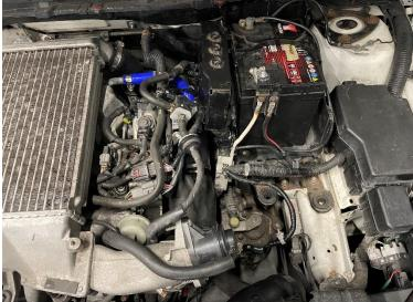
10. Swap the MAF sensor from the old air box to the new housing using the two supplied M4 bolts. Then attach the supplied silicone reducer as shown, with jubilee clips. Also, unwrap the tape securing the MAF sensor wiring from the loom (blue arrow) to allow it to reach further.
