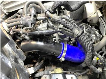
8. Remove the vacuum line disconnected in Step 5 and fit the supplied replacement to the new intake pipe (blue arrows) with cable ties to secure. Then fit the supplied silicone hose to join the intake pipe to the intercooler (orange arrows) with jubilee clips. Then reattach the front hose removed in Step 4 (green arrow).
