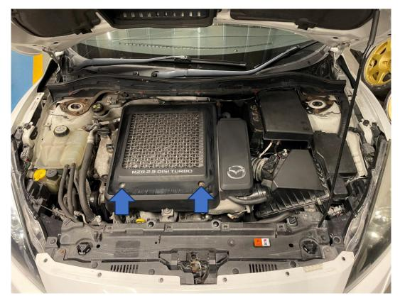
2. Unplug the MAF sensor (blue arrow), then remove the 10mm bolt at the front of the air box (orange arrow) and loosen the jubilee clip at the rear (green arrow). You can then remove the air box from the car by firmly lifting it up off its rubber mountings underneath and manoeuvring past the air feed at the front.
