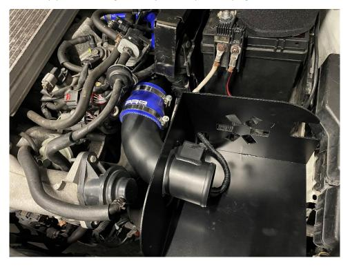
14. Finally, fit the air filter and secure using the supplied jubilee clip. You can then refit the engine cover.
