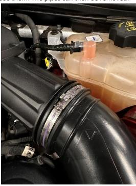
6. Push back the rubber joiners from the air feeds at the front and then remove the original air box from the car by firmly but carefully lifting the corner and pulling it from the rubber mounts. As you remove it, you will need to disconnect a wiring clip on the left-hand side an unclip a small pipe from the right-hand side.
