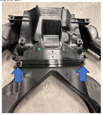
15. Begin to install the supplied upper air guide using the M6x60mm Socket Head bolts with washers and place the supplied spacers between the upper and lower air guides but only tighten the bolts half a turn so that the upper plate is loose to allow adjustment. Then introduce the original air feed onto the rubber joiners and pull it back to allow it to be manipulated into place between the upper and lower air guides.
