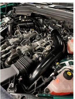
10. Now fit the lower air guide and mounting brackets using the supplied M6x16mm Socket Head bolts with washers, as shown. Then install the new induction pipes using the supplied M6x12mm Socket Head bolts to attach to the brackets to the pipes, but do not fully tighten the bolts at this stage.
