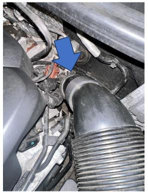
3. To remove the breather take-off, you will need to lift it at the back as you push it outwards. Unclip the other end of the pipework from the turbo inlet pipe and then remove it all together.
