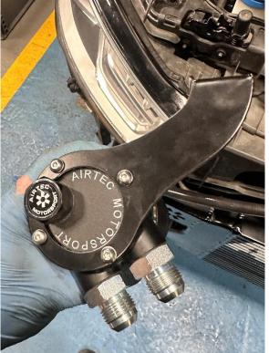
7. Install the bracket onto the car by using the supplied M8 bolt with washer into the spare thread, as shown.
