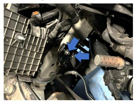
17. With the bracket off, transfer the original rubber bushes to the new bracket, as shown.
