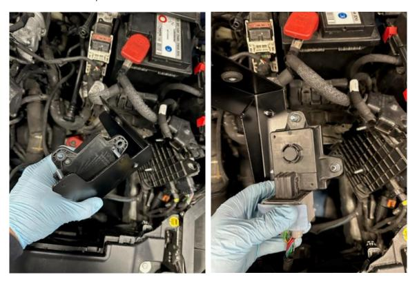
19. Bolt bracket into car reusing the original bolts removed in Step 16.
