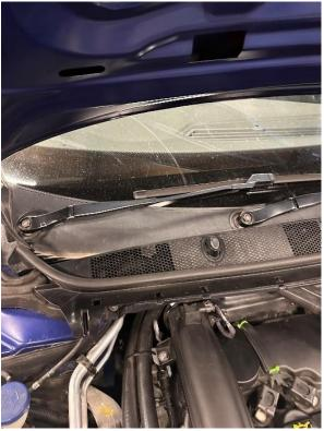
2. Remove the upper scuttle panel by lifting it from the front edge first to release the clips and then pull the panel down and away from the windscreen. Start at one end and work your way across to release the trim. Before the panel can be fully removed, you will need to disconnect the washer jet connection.
