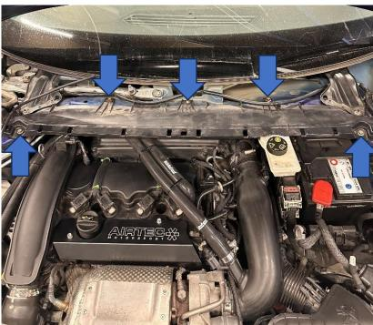
4. Undo the 10mm bolt holding the control box shown and move it out the way to the right-hand side.
