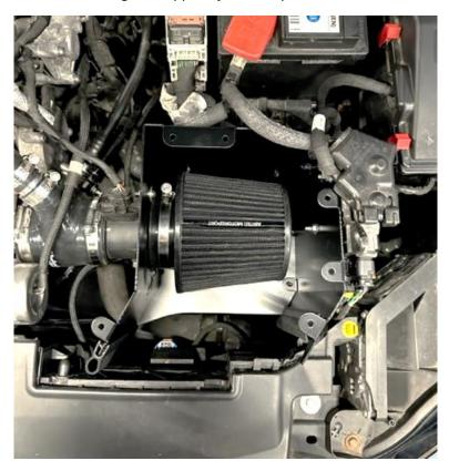
30. Finally, add the induction shield lid with rubber trim and secure by installing the six remaining push fittings into the round holes first and then into the slotted hole last, as this allows for any movement that maybe required. You can then refit the wipers and scuttle panel in reverse of removal.
