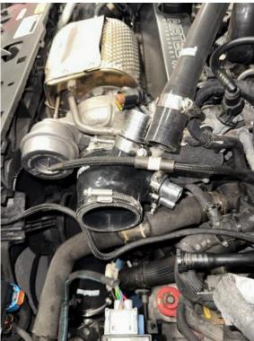
21. Reconnect the two take offs removed in Step 5 by pushing them on until you hear a positive 'click'. The breather hose removed in Step 7 hose can also be reinstalled.
