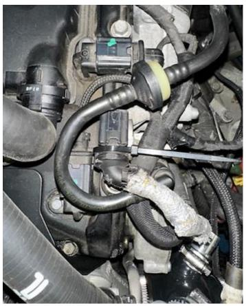
23. Now reinstall the MAF housing removed in Step 10 and reconnect the wiring plug, which should now have enough length. Then secure with the supplied jubilee clip.
