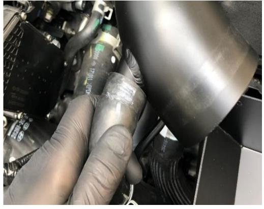
2. Remove the two breather pipe from the intake pipe by squeezing the clips and pull the hoses out of the way.
