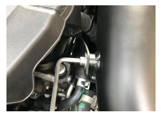
4. Undo the jubilee clips holding the induction pipe to the original turbo elbow and remove the induction pipe from the car.
