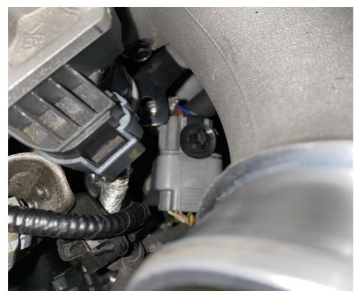
6. Undo the three 10mm bolts holding the elbow to the turbo and remove it. There is a gasket between the two, make sure to not lose this as it will be reused.
