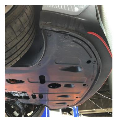
3. In both wheel arches there are three plastic clips that need to be removed using a trim removal tool. There is also a single 8mm bolt higher up that needs removing (orange arrow).
