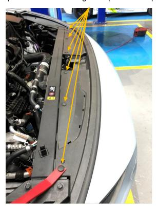
5. The edges of the bumper can now be released, best achieved by gently pulling from the top corner edge where the bumper meets the wing, and then working forward as it pops out. It is advised that another person supports the other side so that once both sides are pulled forward, one person can support the bumper whilst the other disconnects the three electrical connectors left to un-plug: two on the near-side and one on the off-side. The bumper can now be fully removed and put aside safely.
