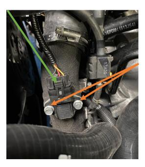
6. Remove the vac line from the takeoff on the pipe by squeezing the clip together and then pulling the hose off and then undo the 10mm bolt holding the solenoid to the pipe. Move out of the way for now.
