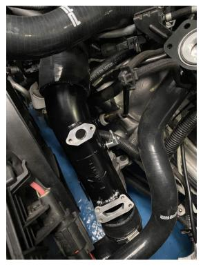
18. You can now build back up the cold side pipe by attaching the MAP sensor to the pipe using the supplied M5 X 12mm with washers, reconnect the plug, attach the solenoid to the mount reusing the original bolt and attach the vacuum line to the take off and secure with the original clip.
