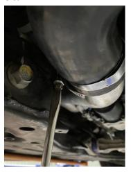
12. Remove the rubber grommet and top hat from the original bracket and insert into your new bracket, attach the bracket loosely to your new larger pipe using the supplied M6 x 12mm hex head bolt and washer.
