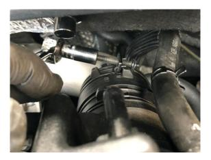
2. Unclip the 2 breather hoses on top of the induction pipe at the back of the engine bay and also the clamp holding on the hose at the front on the induction pipe by squeezing the clips with a pair of pliers and pull the clamp down the hose. The hoses can then be removed by pulling the hoses off the original pipe.
