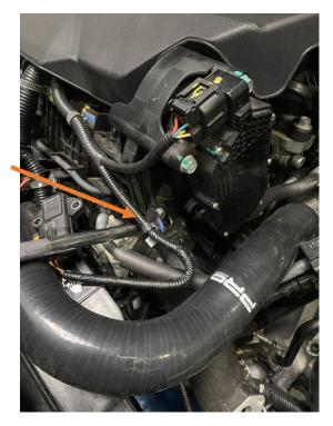
8. From the top you should be able to get access to the hose clip holding the lower silicone to the intercooler, loosen this and then the whole assembly can be pulled out from the car. If you cannot undo this clip from above then undo it after removing the undertray in the following step.
