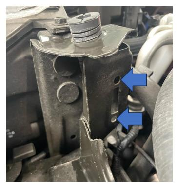
2. Make sure you use the correct sided bracket (please study picture below) and then feed the supplied bolts in from behind, as shown.
