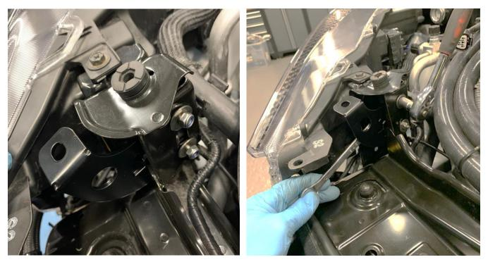
4. Finally, you can now fit the Aero Catch bonnet pin and adjust the angle of the bracket to suit. Once in the correct position and the Aero Catches are fully fitted and aligned, fully tighten the mount's nuts and bolts.
