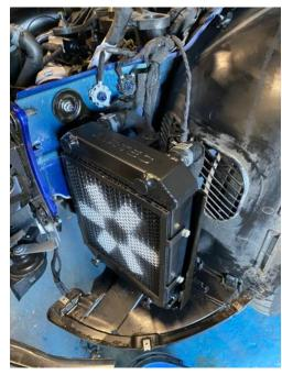
8. Secure the radiator in place using the supplied bolts with washers. You can now refit the ducting by sliding it back onto the mounting pins in reverse of Step 4. The ducts may require minor trimming with a sharp knife to fit squarely.
