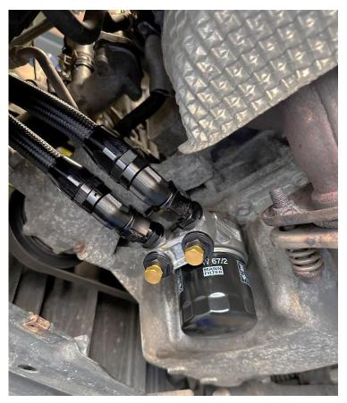
19. Fit the supplied oil line separators as shown to position the lines away from harm's way.
