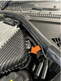
2. Unplug the Map sensor by squeezing the clip as you pull downwards.
