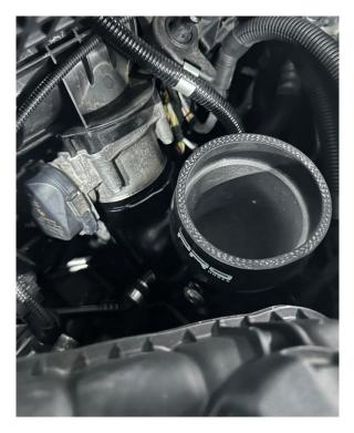
8. Finally, ensure all hose clamps are fully tightened before following Steps 1 to 4 in reverse.
