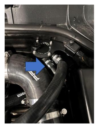
4. Finally, install the 90-degree plastic elbow into the intake pipe, as shown. Then install the silicone hose from the catch can onto the elbow with jubilee clips and tighten.
