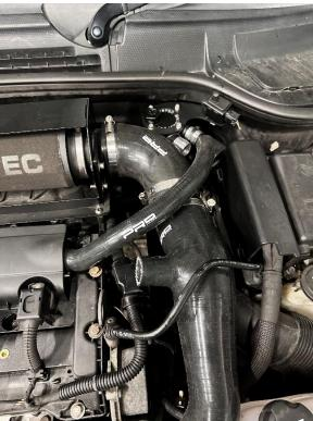
2. Install the supplied push fit connector onto the angled end of the hose, as shown.
